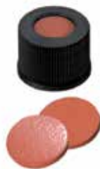
Item No. 13PPS2 13 mm closure PP screw cap with hole black natural rubber red-orange / TEF transparent 60 ° shore A 1.3 mm
