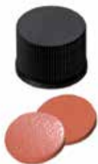
Item No. 13PPS1 13 mm closure PP Black screw closed Natural rubber red-orange / TEF transparent 60 ° shore A 1.3 mm
